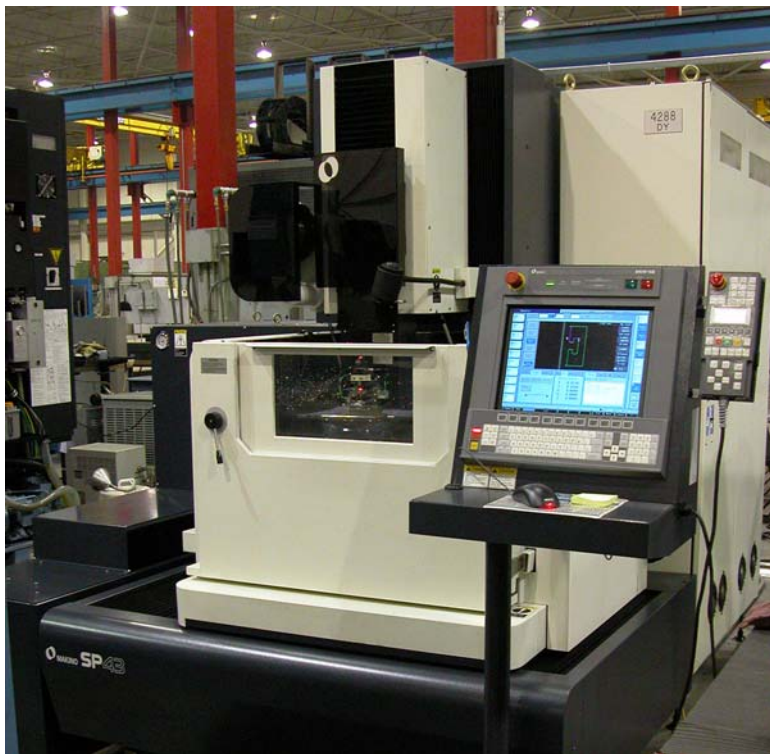
Caption: New Wire EDM machine uses heat technology software.
